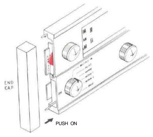
Figure 9. Fitting End Caps To Tuner Panel.
