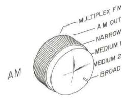
Figure 2. AM Function Switch.
