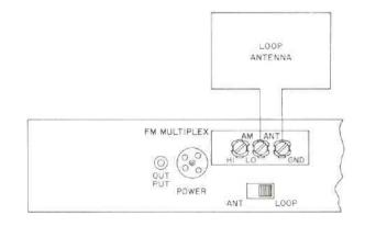
Figure 11. Indoor Loop Antenna Connections.
