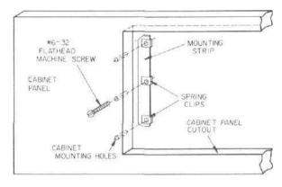
Figure 8. Securing The Mounting Strip To The Front Panel.
