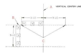
Positions "A" to "C" show the location of the vertical center line, the use of the measuring tool (mounting strip) to locate the horizontal center line, and how to measure off the two points to the right and left of the vertical center line.
