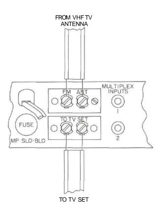
Figure 16. VHF TV Antenna Connections.
