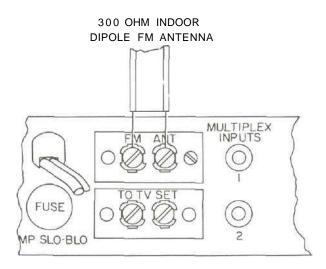
Figure 13. Connection For 300 Ohm Indoor Dipole FM Antenna.
