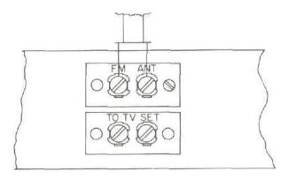
Figure 14. Connection For 300 Ohm Outdoor FM Antenna.
