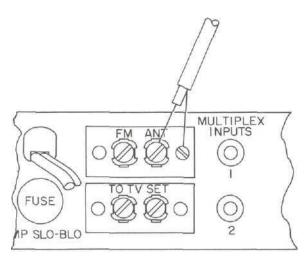
Figure 15. Connection For 75 Ohm Coaxial Antenna.
